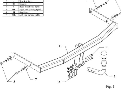
This towing hitch is designed to assembly in following cars: SKODA ROOMSTER, produced since 2006, catalogue no. H16 and is prepared to tow trailers max total weight 1200 kg and max vertical load 75 kg.
